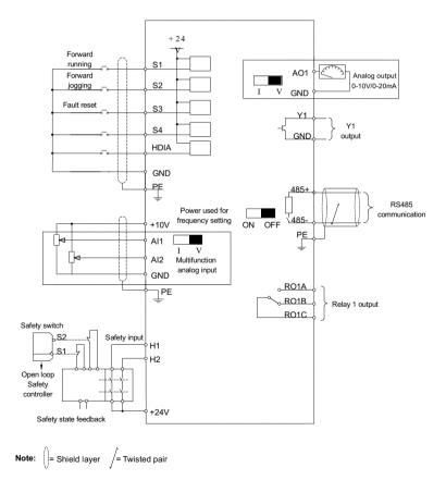
Figure 2-2 Control Circuit Wiring
